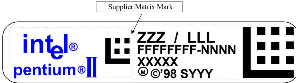
New Mobile Pentium® II Processor in Mini-Cartridge Package Label with Supplier Matrix Mark Removed
