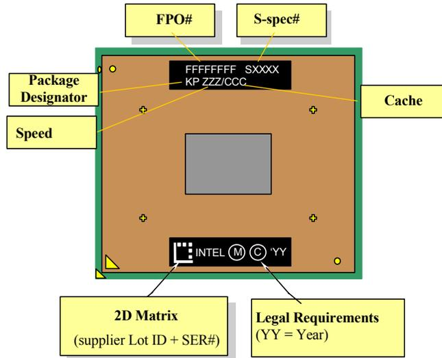
**Mobile Intel® Pentium® II Processor BGA Package Markings**
