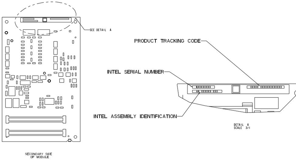
**Intel® Pentium® II Processor Mobile Module with On-Die Cache (MMC-1) Markings**
