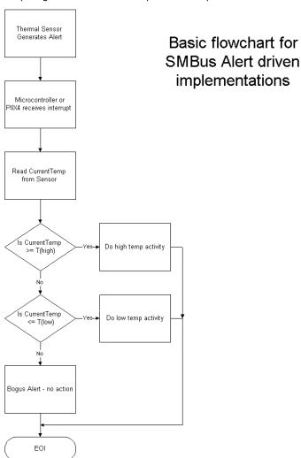
Figure 2. Workaround Flowchart: SMBALERT#-Driven System
