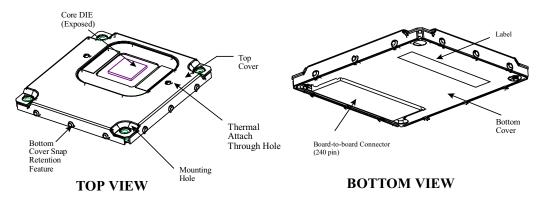
Mobile Intel® Pentium® II Processor Mini-Cartridge Markings
