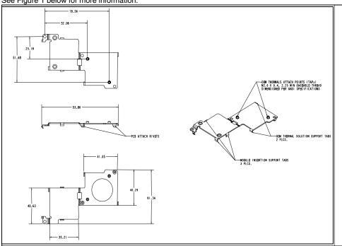
Figure 1. TAP Gageable Thread Clarification
