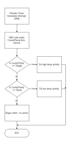
Figure 3. Workaround Flowchart: SMI#-Driven System
